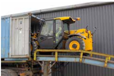
3m forward reach for placement deep inside containers.
