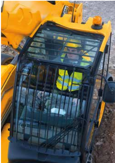
Opt for front and top screen roof guards for added protection from falling objects.
