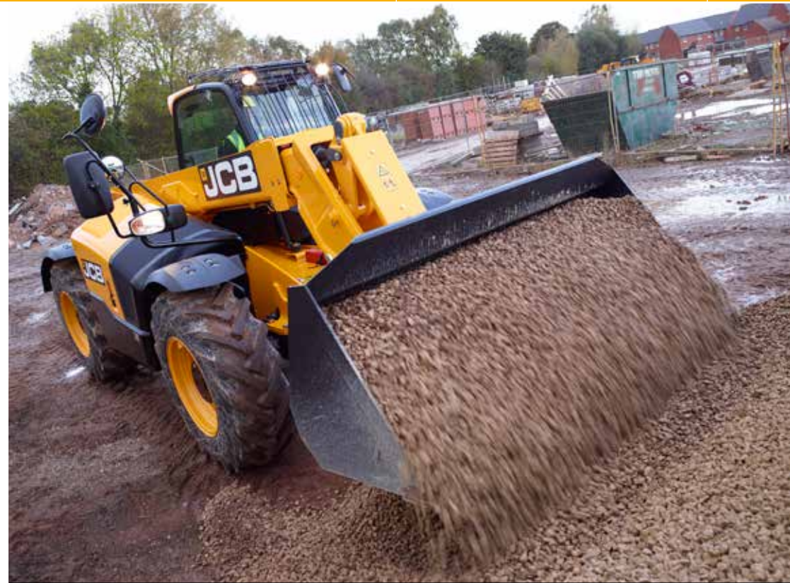
High back-off brakes reduce viscous drag during roading and rehandling which improves fuel economy by up to 2%.
