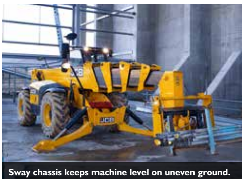
Sway chassis keeps machine level on uneven ground.
