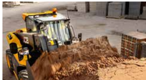
JCB's Adaptive Load Control system automatically prevents overturning forwards during heavy load handling.
