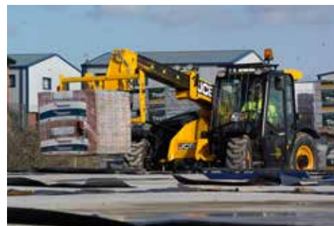
1.25 tonnes lift capacity at full reach.
